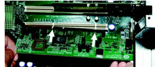
Figure 3-1: Insert the Adapter into the PCI Slot
